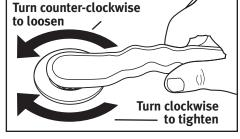
to turn, remove the valve completely and add a small amount of silicon grease to the valve Oring and reassemble.
